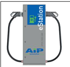
The HPDC 1000/400 consists of a charging station, which is placed near the vehicle in the test cell or soak room and a power unit, which is located near the power control cabinet of the test bench. The power electronics for generating the regulated DC charging voltage is preferably connected to the existing DC link of the motor
