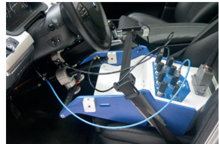
EMC chassis dyno: Optional pneumatic operated EMC type drive robot (AIP P-JAMES)
