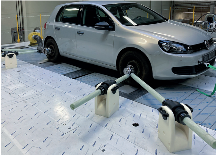
EMC chassis dyno application with EMC type wheel hub 4-WD restraint system
