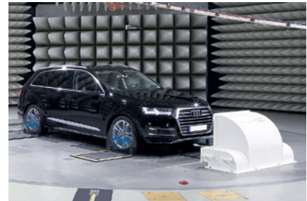
EMC test stand applications: 48° EMC chassis dyno with 11 meter dia. turn table
